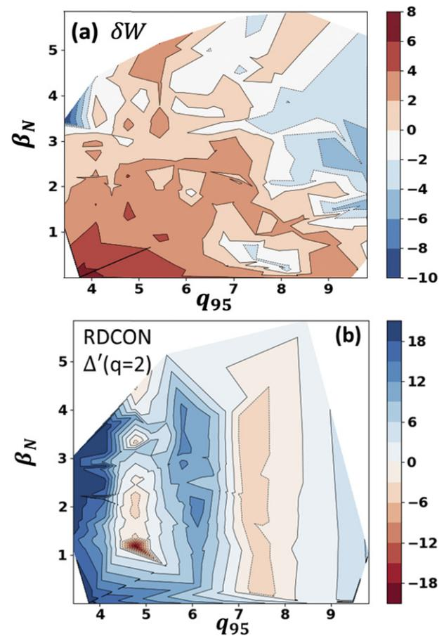
**Figure 1.** (a)  $n = 1$  external kink stability ( $\delta W > 0$ , stable) and (b) 2/1 tearing stability ( $\Delta' < 0$ , stable), as a function of  $q_{95}$  and  $\beta_N$  for a 2 MA, 1 T, 12 MW NSTX-U scenario with  $q_{\min}$  just above unity.
