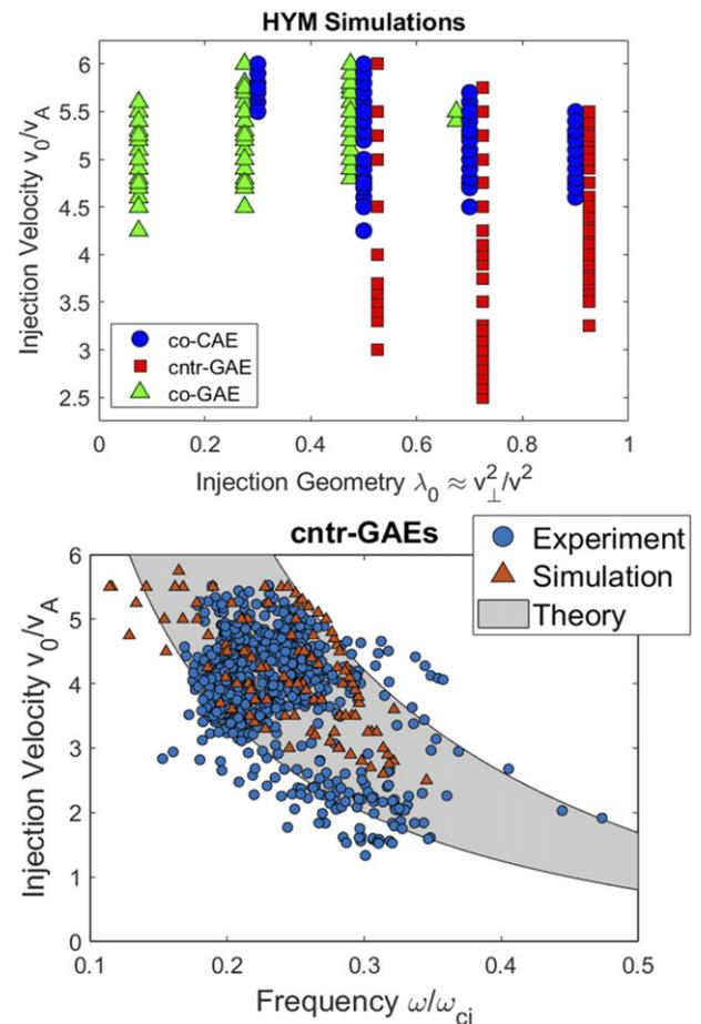
**Figure 4.** (Top) Unstable  $|n| = 3-12$  GAE/CAE modes predicted by HYM as a function of the beam injection geometry  $\lambda_0 \approx (v_{\perp}/v)^2$  and normalized velocity  $v_0/v_A$ . (Bottom) Comparison of experimentally observed counter-GAEs, unstable simulations, and theoretically predicted regimes, as a function of normalized injection velocity and frequency ( $\omega/\omega_{ci}$ ). Reproduced courtesy of IAEA. Figure from [56]. Copyright (2021) IAEA.
