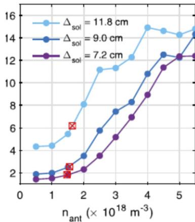
**Figure 17.** Predicted SOL power loss (% of HHFW injected power) vs density in front of the antenna ( $n_{\text{ant}}$ ) and gap between LCFS and antenna ( $\Delta_{\text{SOL}}$ ). Reprinted from [135], with the permission of AIP Publishing.
