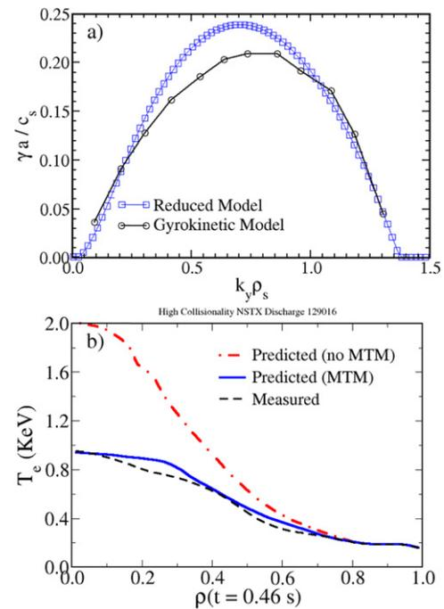
**Figure 6.** (a) Linear MTM growth rates from gyrokinetic simulations and reduced model. (b) Experimental  $T_e$  profiles compared to predictions without and with MTM transport model. Reprinted from [84], with the permission of AIP Publishing.
