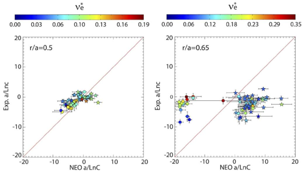
**Figure 7.** Comparison of experimentally measured normalized carbon density gradient vs neoclassical predictions at two different radii,  $r/a = 0.5$  (left) and  $r/a = 0.65$  (right). Symbol color correspond to normalized electron collisionality. Different symbols denote discharges that utilize different between-shot wall conditioning methods: boronization (circles), lithium (stars).
