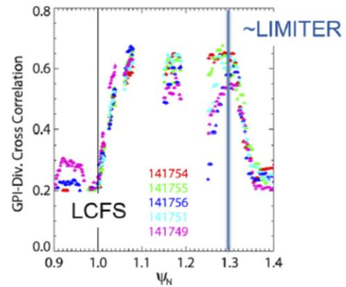
**Figure 13.** Maximum cross-correlation between upstream (GPI) and divertor target (Li I emission) fluctuations, plotted vs  $\psi_N$ . Reproduced courtesy of IAEA. Figure from [111]. Copyright (2020) IAEA.
