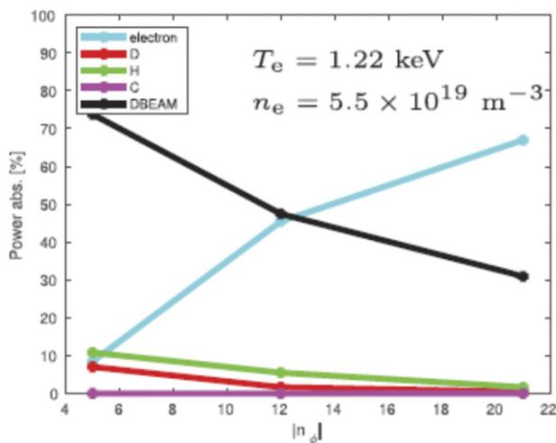
**Figure 18.** HHFW absorbed power vs antenna phasing, assuming 2% H in a full field NSTX-U projection. Reproduced courtesy of IAEA. Figure from [136]. Copyright (2019) IAEA.
