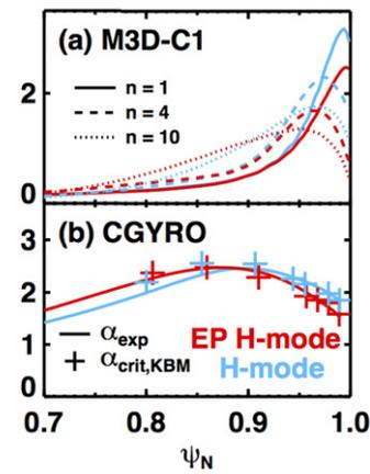
**Figure 9.** (a) MHD kink/peeling eigenfunctions (M3D-C1), and (b) normalized pressure gradient,  $\alpha$ , from experiment (lines) and KBM thresholds (CGYRO, symbols) for both H and EPH mode. Reprinted from [94], with the permission of AIP Publishing.
