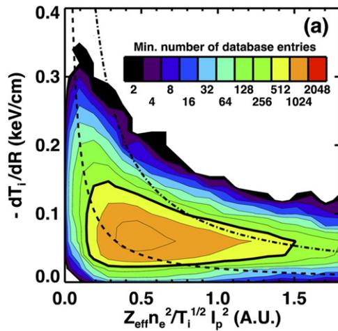
**Figure 8.** (Top). Database of maximum edge  $\nabla T_i$  versus leading order terms of neoclassical transport. Dashed lines represent fixed  $q_{i,neo}$ . Symbols are described in the text. Reprinted from [94], with the permission of AIP Publishing.
