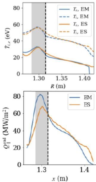
**Figure 15.** (Top) Upstream temperatures and (bottom) target heat fluxes predicted from electromagnetic simulations (Gkeyll) for NSTX-like model SOL. The gray regions indicate the location of particle and energy sources. Reproduced from [119].
