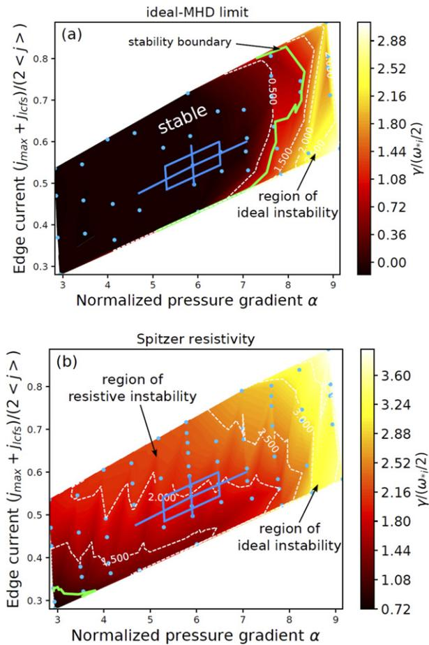
**Figure 10.** Normalized peeling-ballooning mode growth rates vs normalized pedestal pressure gradient,  $\alpha$ , and current density  $j$ , for (a) ideal, and (b) resistive MHD simulations (M3D-C1). Experimental values shown by cross-hairs. The  $\gamma/(\omega_{*i}/2) = 1$  stability boundary is shown by the green lines. Reproduced courtesy of IAEA. Figure from [101]. Copyright (2021) IAEA.
