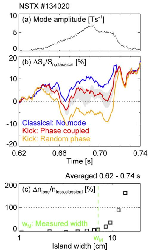
**Figure 2.** (a) Measured amplitude of coupled  $n = 1$  kink + 2/1 tearing mode. (b) Relative difference in neutron rate between simulation and experiment, for classical losses only, or when including kick-model transport from the kink + tearing mode for both phase-coupled and random phase assumptions. (c) Predicted fast ion loss from phase-coupled kink + tearing mode for different tearing mode island widths. Reproduced from [36]. © IOP Publishing Ltd. All rights reserved.
