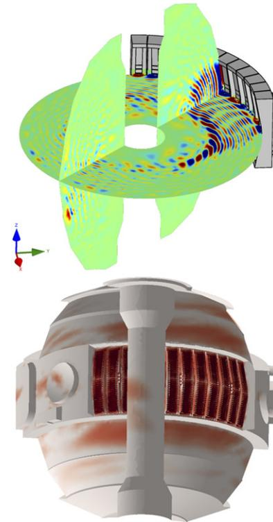
**Figure 19.** (Top)  $E_z$  component of the wave electric field predicted for HHFW heating ( $150^\circ$  antenna phasing) in NSTX-U using 3D Petra-M simulations. (Bottom) Predicted electric field amplitude on the wall surface for  $30^\circ$  antenna phasing where stronger SOL interactions are predicted. Reproduced with permission from [140].
