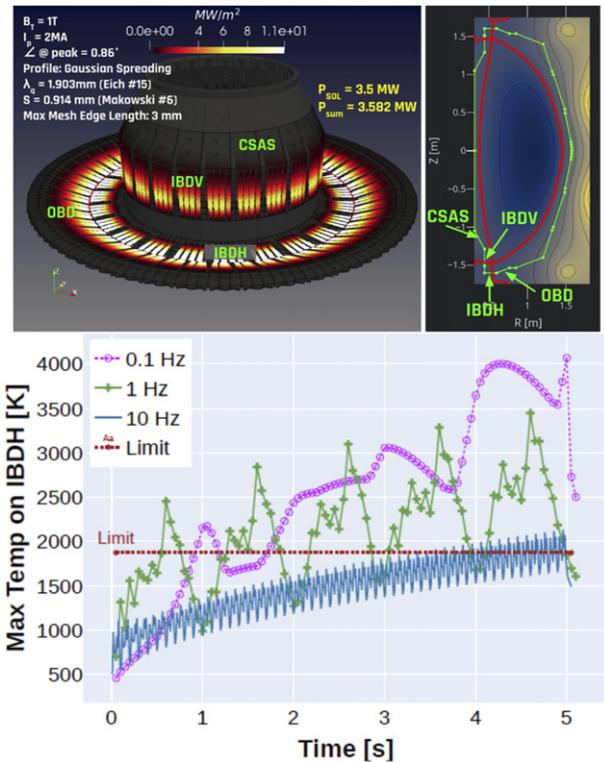
**Figure 16.** (Top) Predicted 3D target heat flux (HEAT) for a full-field NSTX-U projection. (Bottom) Predicted evolution of maximum PFC temperature for different strike-point sweep frequencies. [123], copyright © American Nuclear Society, reprinted by permission of Taylor & Francis Ltd, <http://www.tandfonline.com> on behalf of American Nuclear Society, <http://www.ans.org/>.
