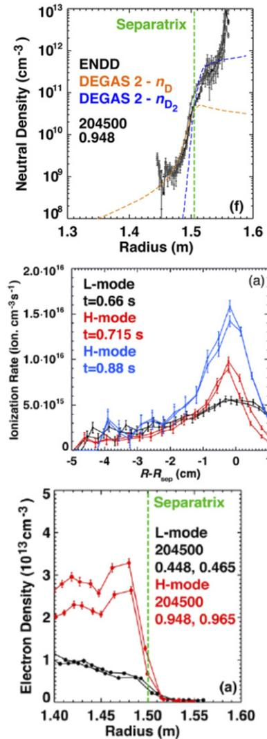
**Figure 11.** (Top) Measured atomic deuterium density compared to atomic and molecular deuterium density from DEGAS 2 modeling for an NSTX L-mode. (middle) Inferred ionization rates (upper-estimate) and (bottom) electron density profile in the edge of L- and H-mode phases of NSTX-U discharge. Reproduced courtesy of IAEA. Figure from [102]. Copyright (2021) IAEA.
