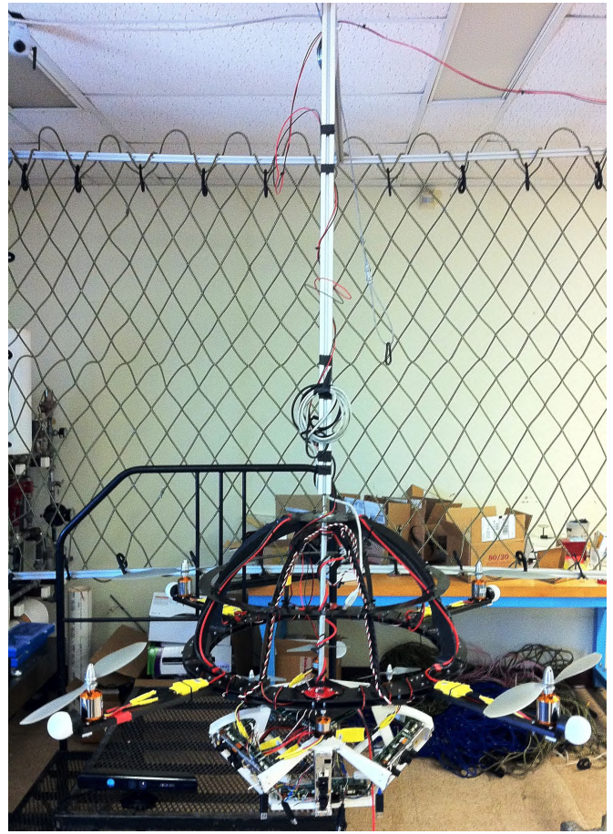
Figure 13: Experimental Setup: The Dual-quad Observer mounted on a vertical bar suspended from the top of a safety cage. Both the flight deck and sensor deck are free to rotate in 3DOF while the vehicle position remains fixed.
