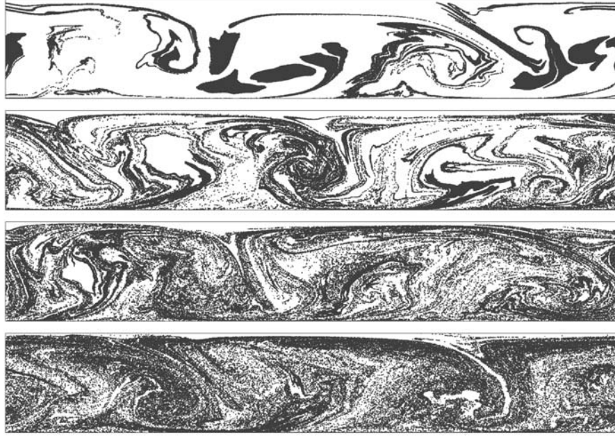
Figure 14. Particle distribution for controlled flow ( Re=10000 , B_0^* = 0.3 , t=47,140,280 )
