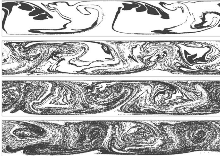
Figure 12. Particle distribution for controlled flow ( Re=6000 , B_0^* = 0.3 , t=47,187,654 )
