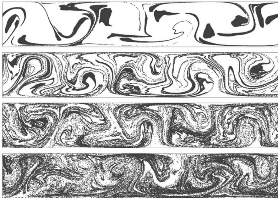
Figure 13. Particle distribution for controlled flow ( Re=7500 , B_0^* = 0.3 , t=47,140,327 )
