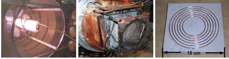
Fig. 3. Left: Helicon source during operation in helium. Center: Cathode source. Right: Copper concentric bias rings mounted on ceramic substrate.
